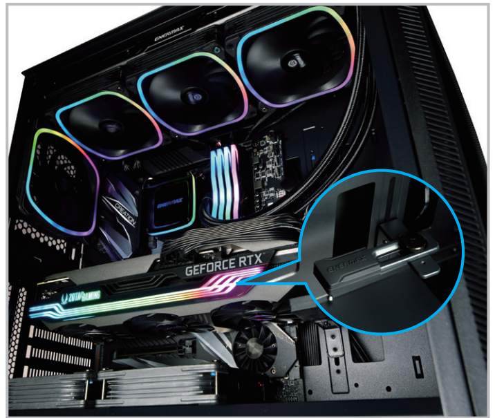
Tool-less GPU Holder
